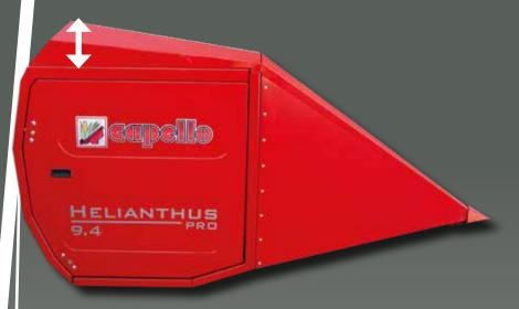
The height of the header sidewalls has been increased to minimize losses and prevent the sunflower baskets from rolling over the edges of the header.
